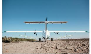
The face of agriculture is changing with aerial drones that will replace the traditional crop duster, with speed, efficiency, and cost benefits, capable of spraying up to 135 acres an hour with one half the cost of traditional spraying, especially valuable for vineyards, which can be dangerous for tractors. Watch the skies for **Pyka** (Silicon Valley) and **Volocopter** (Germany) to take to the skies for autonomous aerial sprayers. (*Progressive Farmer, August, 2020*).
